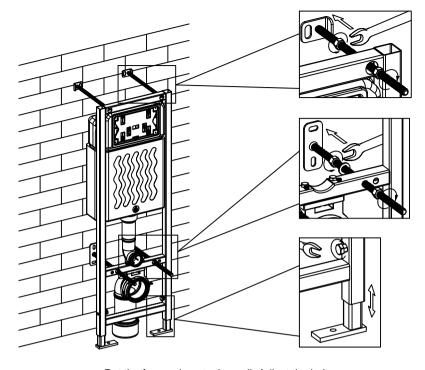
Put the frame close to the wall. Adjust the bolts and adjustable fixing kits to align the frame with the holes on the wall and floor. Then screw the nuts to fasten the frame.
